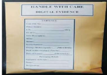
Step 4: Place in inner clothing/ laminated paper envelope. Fill information in self-adhesive labels and affix on envelope along with instructions.
